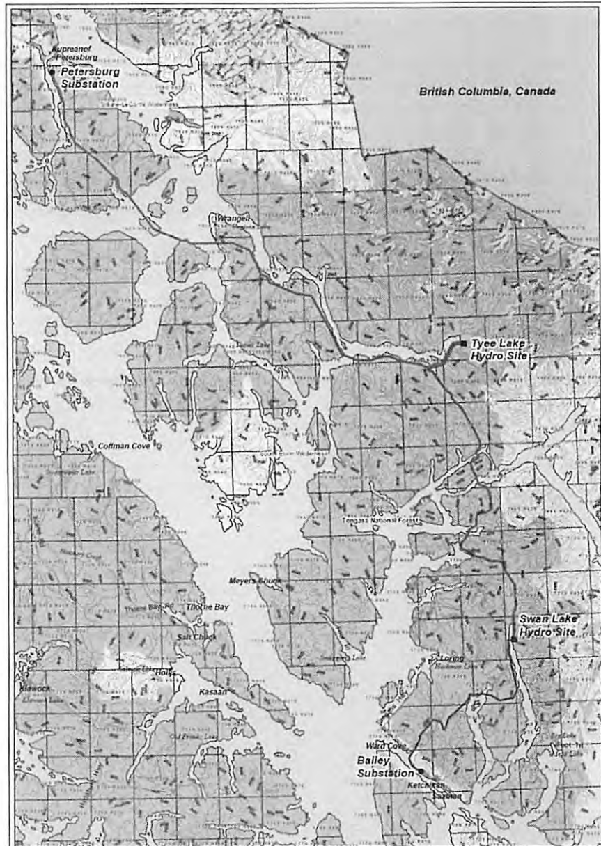
Figure 2- SEAPA transmission from Ketchikan to Swan Lake is shown as blue, Swan Lake to Tyee Lake as red, and from Tyee Lake to Wrangell and Petersburg as purple. SEAPA hydro generation is located at Tyee Lake and Swan Lake with additional hydro generation owned and operated by Petersburg and Ketchikan.
