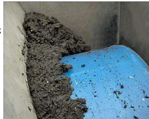
Dewatered dry solids conveyed into the ÖÜÿÔCSÒÁÛÜÒÙÙ discharge section
