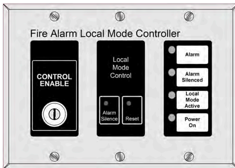
Figure 2: Local Mode Controller Module
