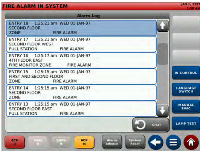
Figure 11: Alarm History Log
