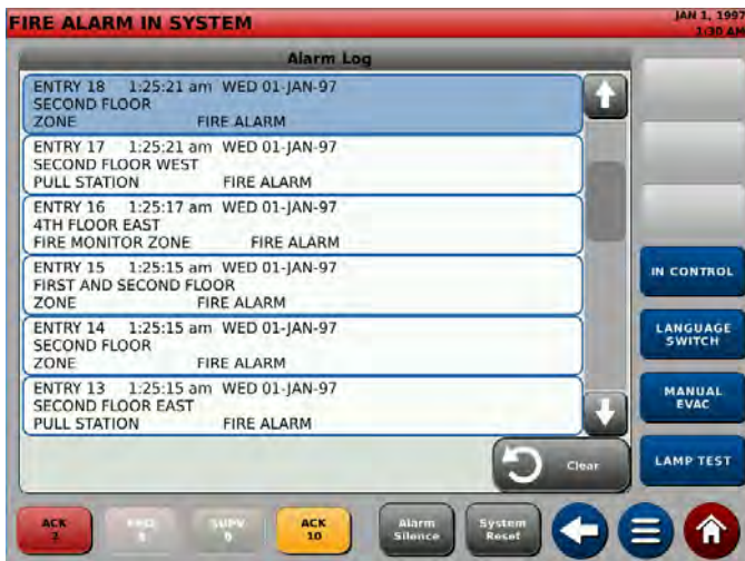
Figure 6: Alarm history log
