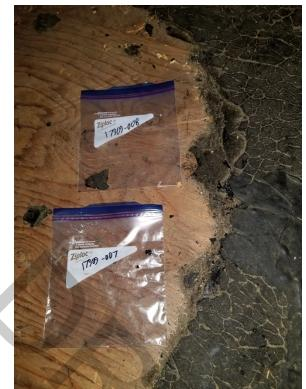
Photo 1: Roofing material of the original building roof is ACM. (May 22, 2018)
