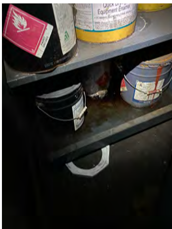
Photo 23: Looking at leaking containers inside a flammable storage cabinet on the mezzanine of the main shop structure.
