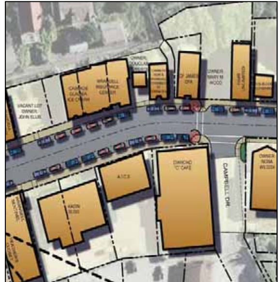
Section of proposed design for Front Street showing parallel parking and bulb-outs
