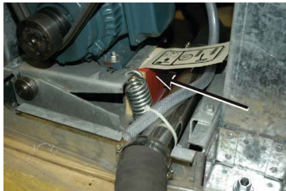
Figure 4: Motor Mount Blocking
