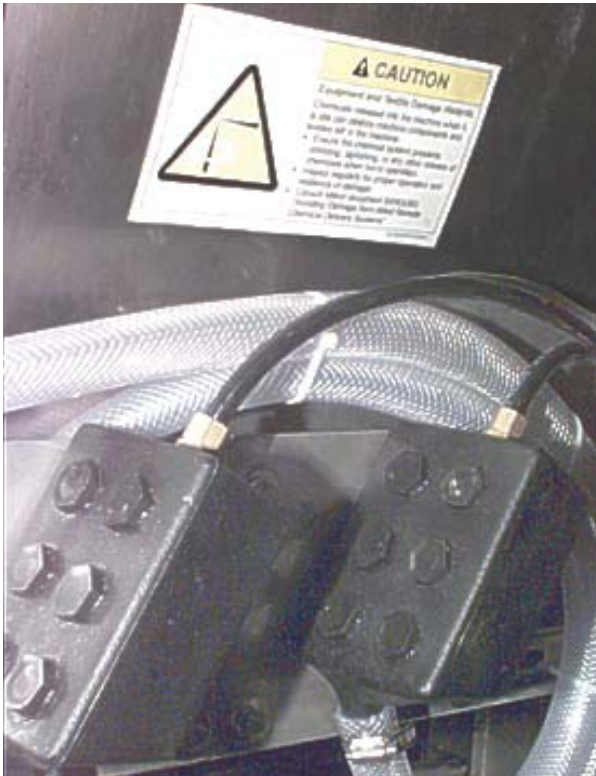
Figure 1: Pumped Chemical Inlets on CBW Batch Washer
