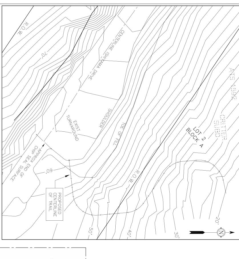
MAXIMUM STUMP HEIGHT INSIDE CLEARING LIMITS IS 0.5 FT. STUMP INSIDE CLEARING SHALL NOT RISE ABOVE THE LEVEL OF THE TRAIL FINISH SURFACE; 9.8' ERTICAL CLEARING LIMIT
