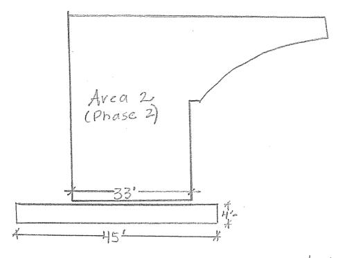
Replace 45' of concrete sidewalk and curb Widen curb cut by five feet (5') to the east side of the opening. Cut at existing joints and provide minimum SIX feet (6') of sloped sidewalk. Match existing slope. 6" thick sidewalk and curb.
